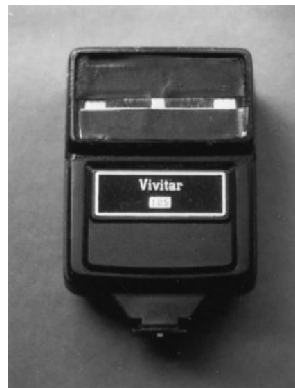
FIGURE 13–12. Camera flash attachment for afterimage test.
